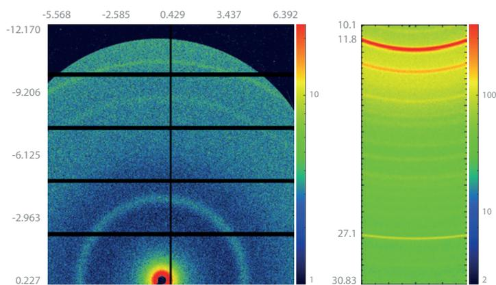
Fig. 1 - 2D SAXS (left - PILATUS3 R 1M detector) and WAXS (right - SWAXS module) patterns from a block copolymer sample obtained at  $d_{SD \text{ SAXS}} = 569 \text{ mm}$ . Exposure time = 10 min. Axis unit =  $q \text{ [nm}^{-1}\text{]}$ .
