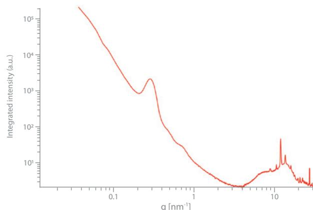
Fig. 2 - Scattering curve from a block copolymer sample resulting from simultaneous SAXS/WAXS measurement at  $d_{SD \text{ SAXS}} = 569 \text{ mm}$ . Exposure time = 10 min.
