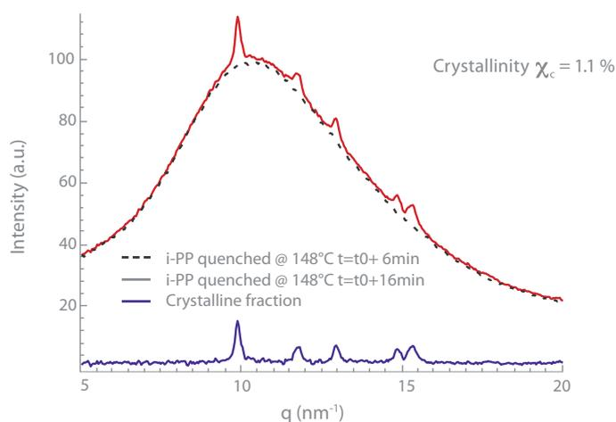
Fig. 1 -1D scattering curves and estimation of crystalline fraction. Time exposure = 200 s
