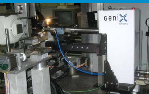
Fig. 1 : The GeniX mounted in the High Pressure Diffractometer present at the High Pressure Facility at LENS
