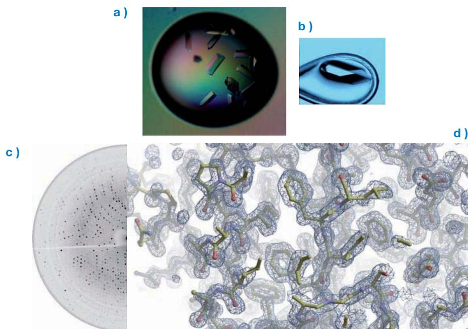
**Fig. 2 : From the crystal to the structure. Photos represent from top left to bottom right : a) a drop b) a trypsin crystal in a loop c) a diffraction pattern measured with GeniX 3D d) an electron density map computed with the recorded data**
