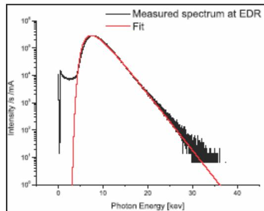
**Figure 2:** Typical spectrum of the primary beam at EDR measured in single bunch mode. The constant intensity at low energy is due to a detector artifact.
