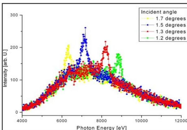
**Figure.1:** Energy spectrum behind the FOX mirror during alignment for different angles of incidence. The spectra were measured from air scattering 90 degrees with respect to the beam direction. The shown spectra are not corrected for air attenuation and the energy distribution of the bending magnet.
