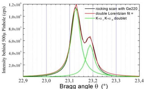
Graph 1: Rocking scan characterisation of the mirror beam (500  $\mu\text{m}$  exit) with a Ge220 crystal on the sample goniometer.
