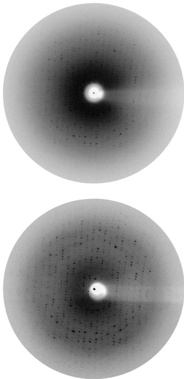
*Fig. 2 : Diffraction images acquired using the Helios optic (top panel) and the FOX2D CU 25\_25P optic (bottom panel) for the same crystal under identical orientation, and with the same grey-scale.*
