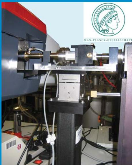
Fig. 1 : Laboratory setup : Microstar Rotating Anode - FOX2D CU 25\_25P – MAR345.
